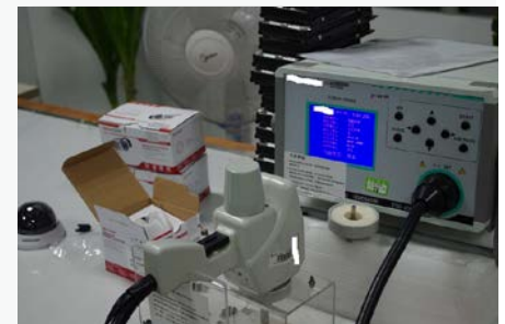
Test device for electrostatic discharge anti-interference
