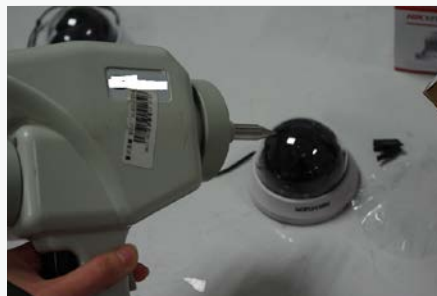
Test device for electrostatic discharge anti-interference
