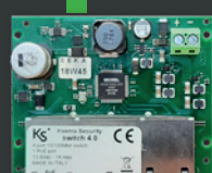
KS-LARES 4.0 SWITCH 4 ports 10/100Mbit
