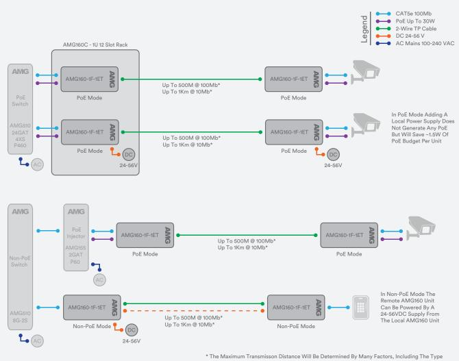
And Quality Of The Cable, Voltage Level Of The PoE Source, Size Of PoE Load etc. For Help & Assistance With Distance Specification Please Contact The AMG Technical Services Team.
